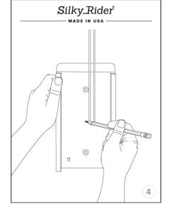
With your other hand get the "Rail" and put it on the wall with face up position where the pen which is into the loop is against it.
