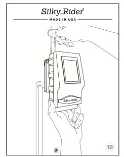
Hold the cord in its position, then join the "Main Device" to the "Rail".
