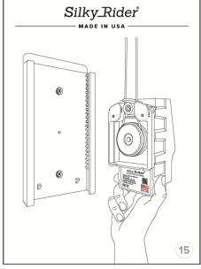
Fix the loop of the curtain cord around the "Big Pulley" which is in the "Main Device" and pass the loop through the "Head System"
