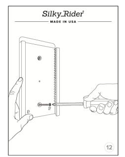
Install the "Rail" using the two screws which have come in the screw pack.
